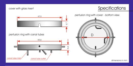
For the use with "35" Petri dishes with an outer diameter of 32.8 mm up to 34.5 mm.
