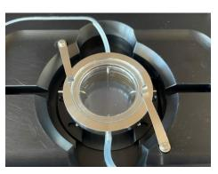
Petri dish "35" with perfusion ring and cover insered into the Heating Insert P 2000
