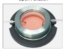
**Observation area**:  $6.6 \text{ cm}^2$ ,  $\varnothing 29 \text{ mm}$
